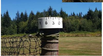
The pelorus is oriented to Magnetic North, so when you take a bearing, it is actually a magnetic bearing that you can follow with a compass (add 20 to get a true bearing).
